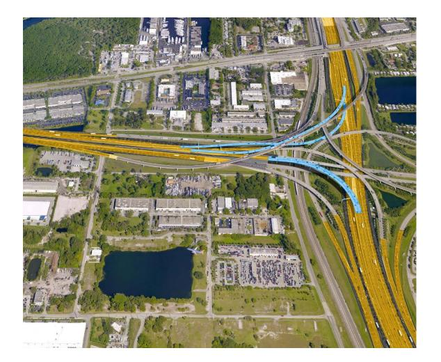
The ramps highlighted in blue depict the ultimate configuration for the I-95 and I-595 Direct Connector ramps
